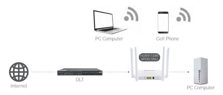
Figure: HUR4113XR Application Diagram
